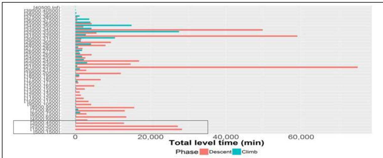
For what they consider in the use of CDO, Brussels Airlines focusses on what happens in the last 100NM before destination, on slopes between 2,7° and 3,3°. This is Brussels Airlines' main KPI. Other criterium to check the descent could be the average rate of descent. For example, in 2018, the average rate of descent from the cruising level into BRU was of 1133ft/min whereas their best profile from cruising level to the threshold would be of 1500ft/min.
