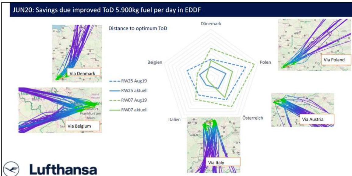
In addition, he said that an enhanced collaboration with DFS led to fuel savings, with the provision by DFS of expected altitudes over specific waypoints, enabling a better management of the vertical profiles. See examples below.
